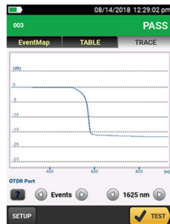
Splitter as seen on an OTDR trace
